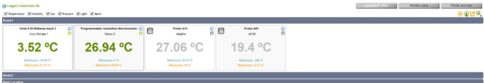
You can check independently temperature, humidity, gas, pressure, light, conductivity generic amp, generic volt, electrical consumption and power levels.
